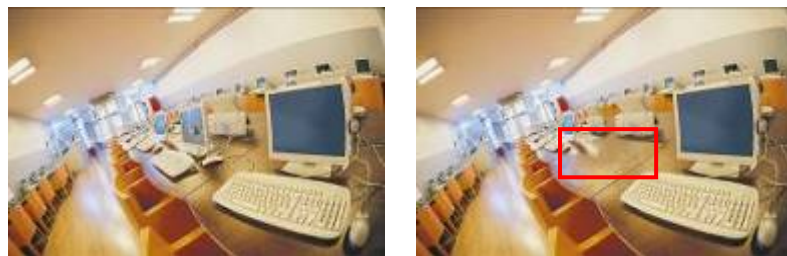
On-board analytics can detect meaningful changes in sequential video clips and trigger alarms. In the scene pictured above, a PC has been removed from the
